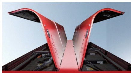
Alloy roof battery cover with wider opening angle
