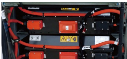
Wire harnesses are protected in layers with high-standard insulation sleeves
