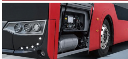
Side cabin door with 160 degree opening angle
